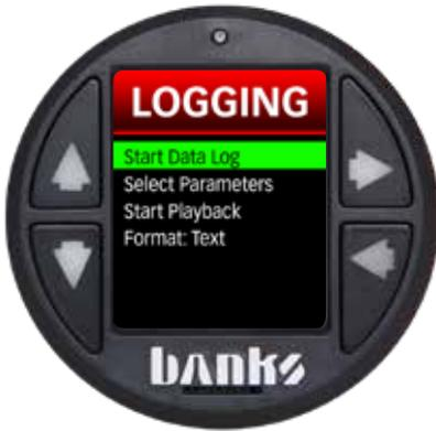
Data logging saves (\*.CSV files) to the Micro SD card. The card must be inserted into the slot in the iDash for data logging to function. Each time the data logging function is turned off, a new CSV file containing the recorded data will be saved onto the Micro SD card. Up to 100 parameters can be recorded at the same time but as the number of recorded channels is increased, the recording rate will decrease, so only record the parameters you need.
