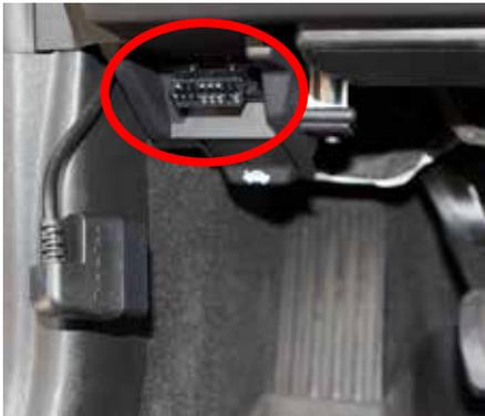
4. Locate the Banks OBDII Cable (See **Figure 3**) and connect the Banks OBDII connector to the vehicle's OBDII port. See **Figure 4**.
