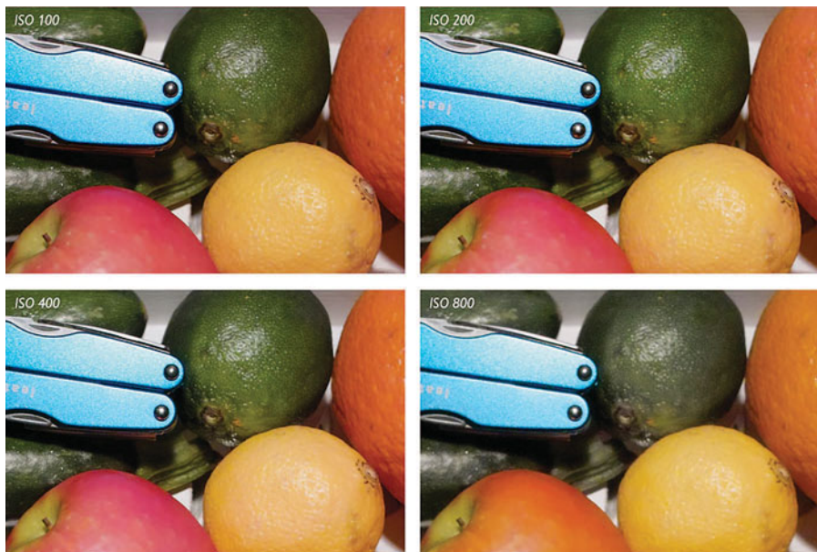
PLATE 5. As the Foveon sensor's light sensitivity is amplified, the images it records exhibit color shifts. Taking the ISO 100 image at top right as a baseline, by ISO 400 red shifts toward yellow, and green both shifts toward cyan and desaturates slightly. At ISO 800, red shifts even farther toward yellow, and green desaturates almost entirely.
