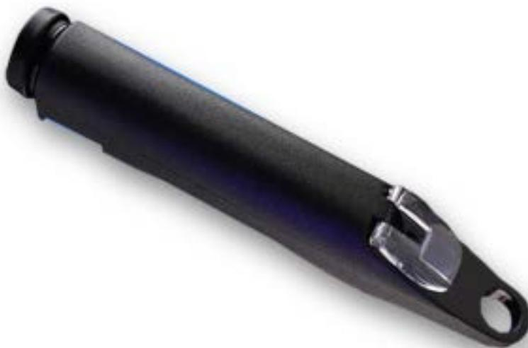
There are many cheap testers on the market, some costing less than cheesburger. We prefer a refractometer for accurate measurements. This precision measurement device will last a lifetime with careful use. It measures freeze protection of ethylene and propylene glycol coolants, and the specific gravity of battery acid, as an added bonus.
