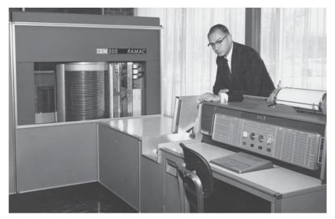
Figure 2.7 IBM 305 RAMAC with 350 magnetic disk drive unit, 1956. Courtesy of IBM Corporate Archives, Somers, New York.
