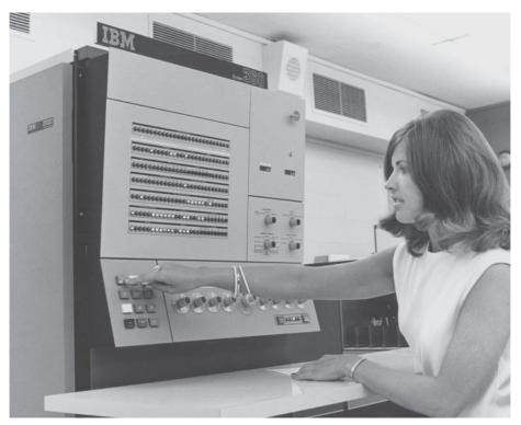
Figure 2.12 Eliot Noyes and Associates and IBM, System/360 Model 40, 1964. View of operator's control panel. Courtesy of IBM Corporate Archives, Somers, New York.
