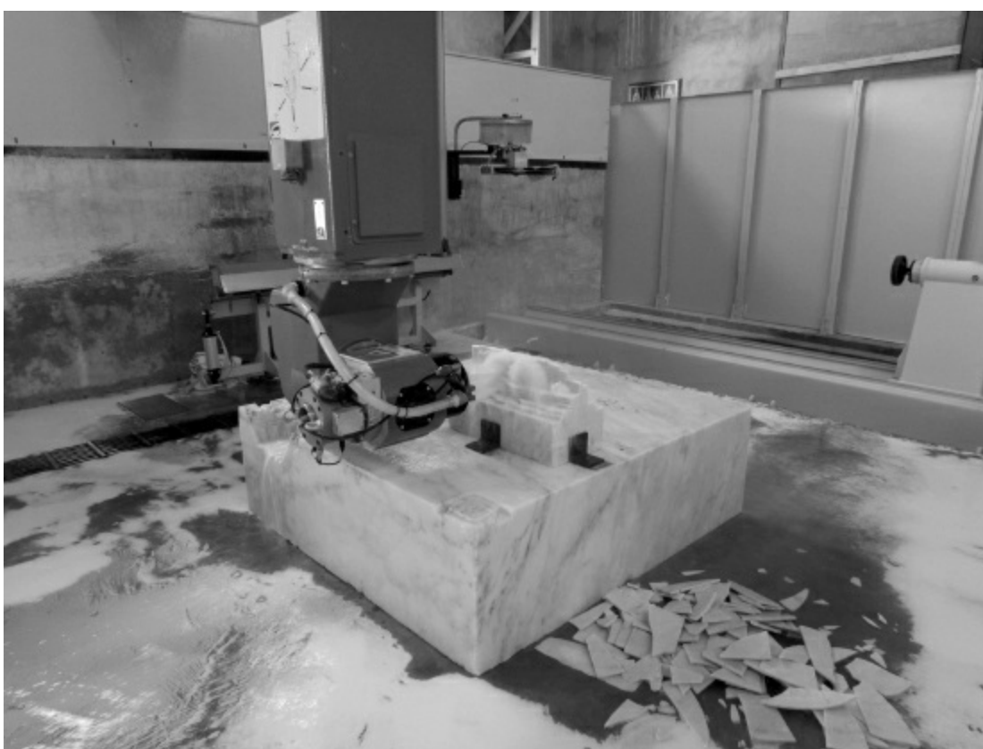
Figure 11.6 Carving by CNC machine. Photograph: Megha Chand Inglis
