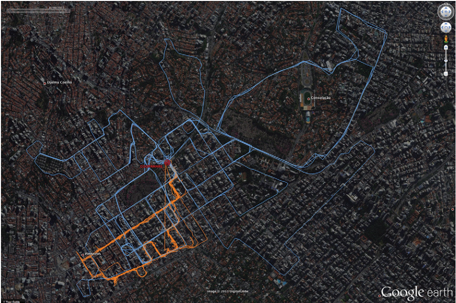
Figure 4.2 Collected GPS traces of COOPAMARE collection routes. In blue, the collection truck routes, in orange, the manual cart collection routes. São Paulo, November 2011. DigitalGlobe, reproduced under Google Maps fair-use policy; courtesy MIT Senseable City Lab 2011.
