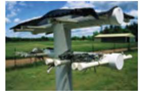
Lichens as air quality indicators used to monitor pollutants, such as mercury, at the Mercury Monitoring Station of the Wisconsin Department of Natural Resources.
