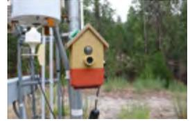
Monitoring station with Bird Box Cam as part of the CENS testbed, the University of California James Reserve.
