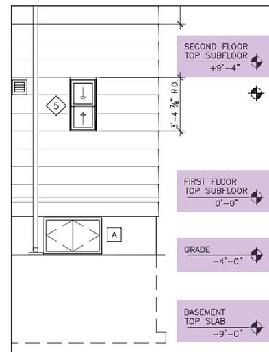
Elevation tags indicate distances between floors, based on the height of that point above or below the first floor
