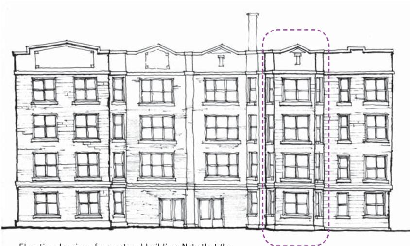
Elevation drawing of a courtyard building. Note that the angled side windows of the bay windows appear narrower because they are not perpendicular to us.
