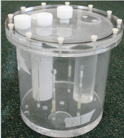
Simulation using GATE 3.0.0 modeled the contrast phantom shown. Isotope simulated was ^{124}\text{I} .
