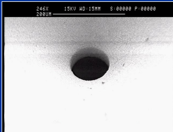
Image of 100 microns pinhole
