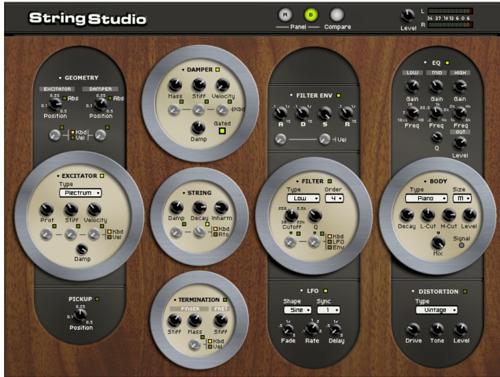
Figure 9: Synthesis modules of String Studio (Panel B).
