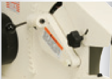
BELT TENSIONING ADJUSTMENT
