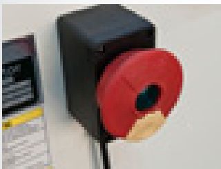
ON/OFF WITH SAFETY KEY
