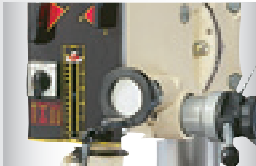
FINE FEED ADJUSTMENT KNOB IN EASY TO REACH LOCATION
