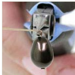
Step 4 Using your round nose pliers, grasp the wire right at the bend.
