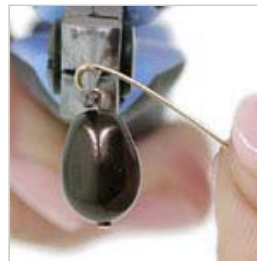
Step 5 Pull the wire around the round nose pliers until it is almost pointing directly down.
