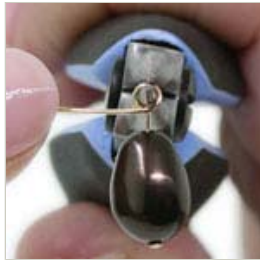
Step 7 Continue pulling the wire around the nose of the pliers until the loop is completely round.
