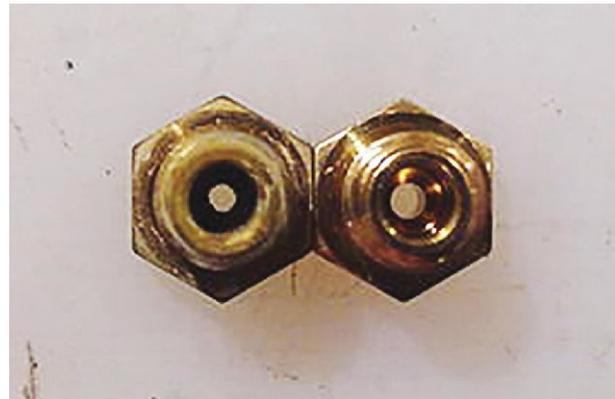
Figure 2: Restricted jet on left, normal jet on right.
