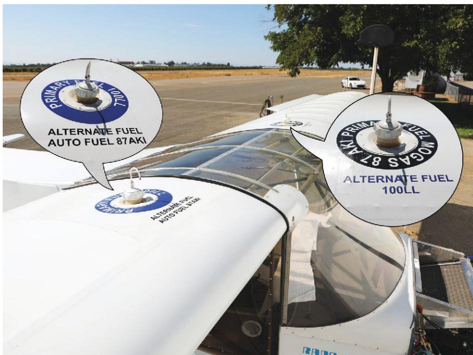
**Figure 3:** Rans S-6S Coyote II right and left fuel tanks.
