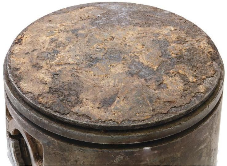
**Figure 2:** Close-up of lead build up on a Rotax Piston.
